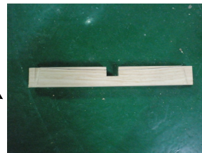
An accomplished transverse groove for a lap joint
